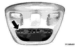
Use this button to change the display from U.S. to metric measurement units.
